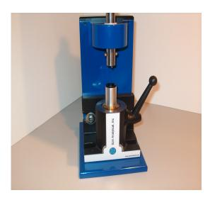
Figure 3: Insertion of cell housing
